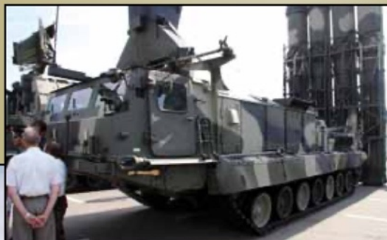
◀▲ 9A83 TELAR (Transporter Erector Launcher And Radar)
